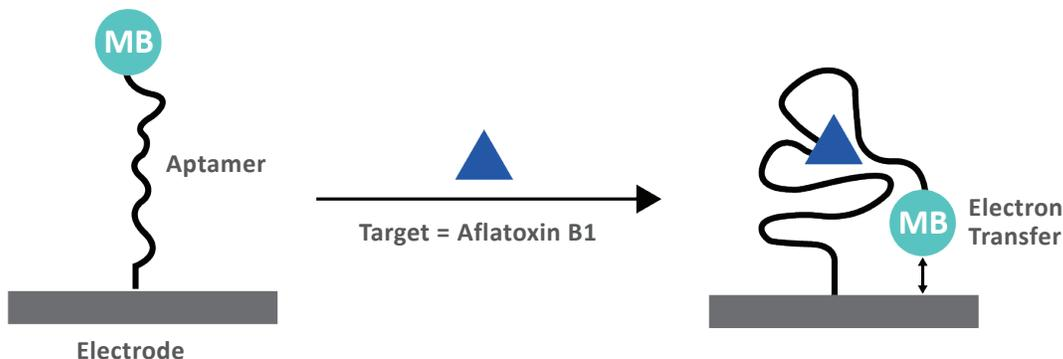
*Figure 2. Aptasensor for Aflatoxin B1 Detection*
